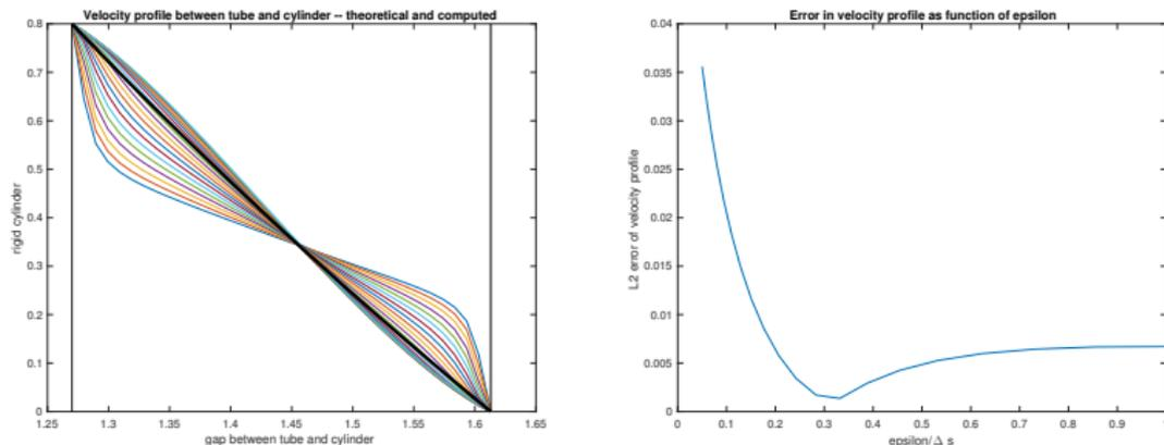
**Figure:** The velocity profile between an infinitely long rigid cylinder of radius  $R_c$  and an infinitely long rigid tube of radius  $R_t$  is  $u(r) = \frac{U(\ln(R_t) - \ln(r))}{\ln(R_t) - \ln(R_c)}$ . This is compared with the velocity computed using the method of regularized stokeslets with varying values for  $\epsilon$ .
