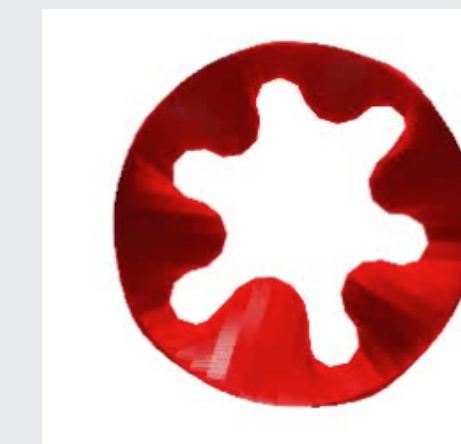
Figure 5. Tube (viewed from end) deforms with circumferential wave number 6 after buckling due to pressure drop.
