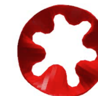
Figure 6. Tube (viewed from end) deforms with circumferential wave number 6 after buckling due to pressure drop.
